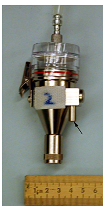
Fig. 9.11. GK2.69 cyclone. May be used as a thoracic or respirable sampler
